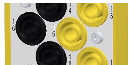
Figure 3: Close up view of the 'finger safe' test plug sockets that accept standard 4mm shrouded test plugs
