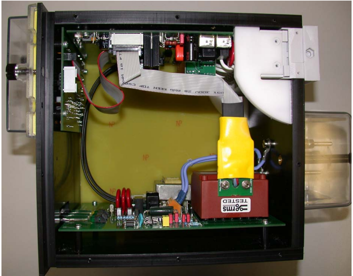
3A300 top view with cover removed showing the connection between the blue pilot wire side PCB and the isolated side PCB using optical fibre links & isolating transformer (Bottom right).
